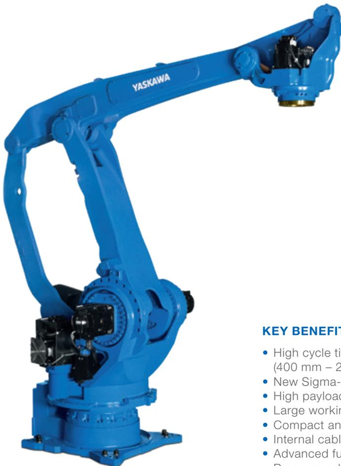
With over 1700 cycles per hour, the fast and powerful 4-axis MOTOMAN PL190 robot offers top performance for box, carton and bag palletizing for end-of-line packaging and logistics applications.
